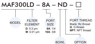
Blank: PC bowl Blank: Standard type (Semi-auto drain)
